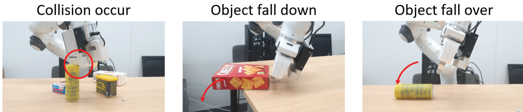
Figure 4.17: The representative examples of the failure cases for pushing manipulation.
