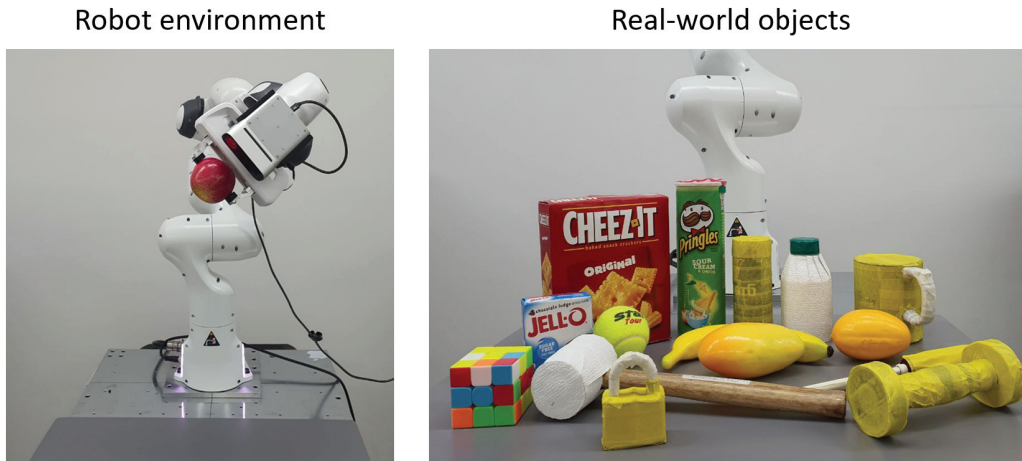
Figure 3.7: Robot manipulator equipped with the vision sensor (left) and real-world objects used in the grasping experiments (right).
