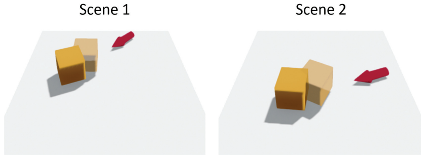
Figure 1.1: The box object and pushing vector in Scene 1 are transformed by some same planar rigid-body transformation as those in Scene 2 . An ideal pushing dynamics model should be SE(2) -equivariant, i.e., the resulting motion in Scene 2 is a transformation of that in Scene 1 .
