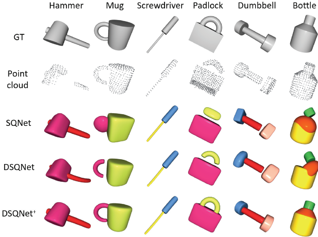
Figure 3.13: Shape recognition results for SQNet, DSQNet, and DSQNet + for six types of multi-part objects in object dataset.
